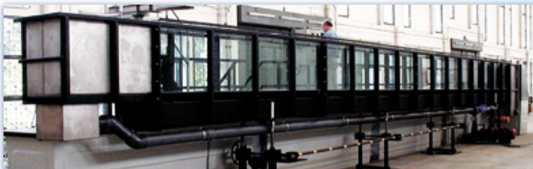
HM 161 Experimental Flume 600x800mm Experimental sections for performing flow experiments in open flumes of 16m length, closed water circuit and inclination adjustment
