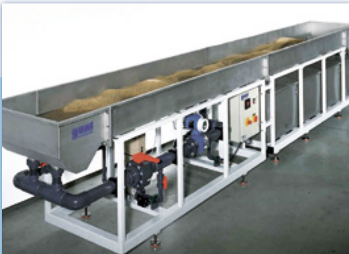
HM 168 Sediment Transport in River Courses Investigation of sediment migration with and without structures
