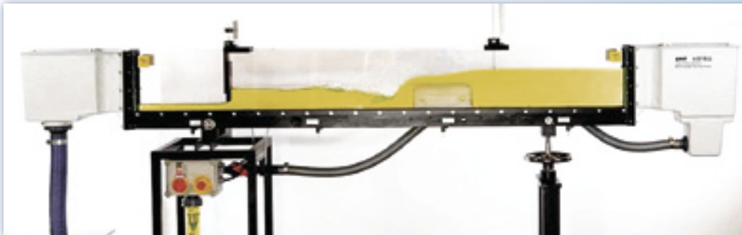
HM 160 Experimental Flume 86x300mm Experimental section for performing flow experiments in open flumes with lengths of 2,5m or 5m available, closed water circuit and inclination adjustment
