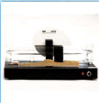
HM 166 Fundamentals of Sediment Transport Investigation of the movement of sediment in flows
